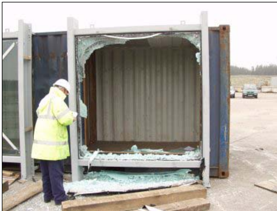
P11: Test specimen 2R-1 post detonation of ***kg TNT @ 16.75m.
